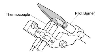
Figure 18 - Correct Pilot Flame Pattern
